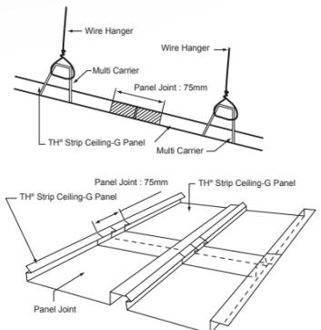
Typical Detail Joint using Panel Joint
