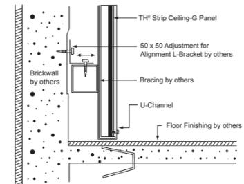
Typical Detail at Bottom TH® Strip Facades to Floor
