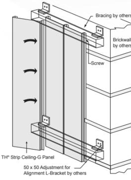
Typical Installation Detail TH® Strip Facades with Multi Carrier
